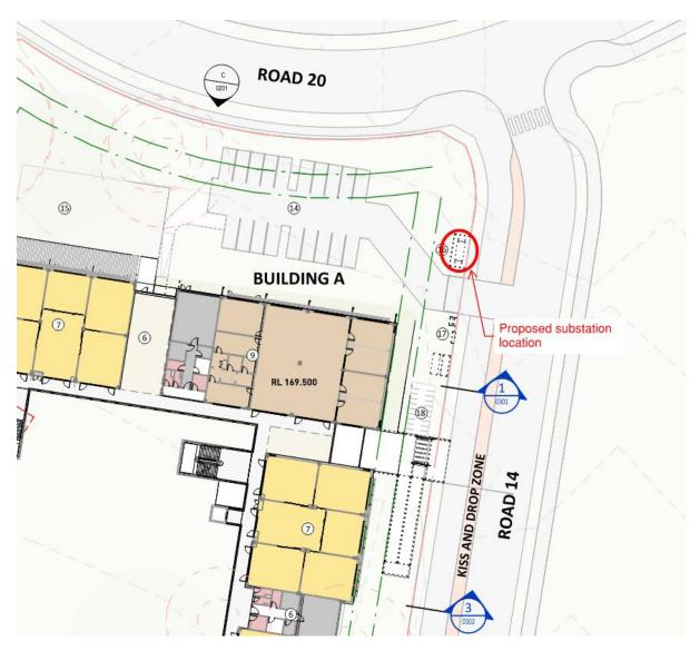
Figure 5: Proposed Substation location (located with the undnerstanding that incoming high voltage cabling is installed on 'road 14').
